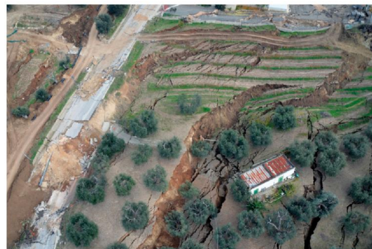
Montescaglioso landslide (Italy – 2013), following extreme rainfall over a stabilized paleo-landslide body (Lazzari et al., 2018)
